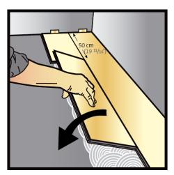
Once first two rows are installed, ensure expansion gap between walls and boards are shimmed securely.
