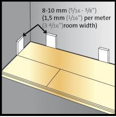
Start with tongue side facing wall and long groove side directly up against straight edge. Spread adhesive enough to cover one board width. Use only as much adhesive as can be used during manufacturer's open time of adhesive.
