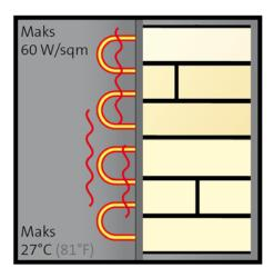
With a thermal resistance of 0,15 W/sqm, the 14mm, multi-layer hardwood flooring is suitable for gluing to a sub-floor which incorporates an under-floor heating system. The heating effect must not exceed (60W/sqm). The surface temperature of the hardwood flooring must not exceed 81°F (27°C). The heating system must distribute the heat evenly throughout the entire floor irrespective of the heat setting.
